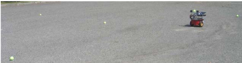
Fig. 9.2. The Pioneer 3DX rover on the test field. The tennis balls laid on the ground are used as reference points for the estimation of a ground-truth rover position independent from the visual odometry algorithm
